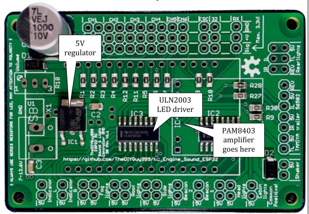
Note, that the LED need to be wired "common positive". This means, that the long LED legs (the + side) can be wired together, using a **shared 5V** potential. The negative side of each LED (the short wire) needs to be wired to an **appropriate current limiting resistor** and then to the LED output pin.
